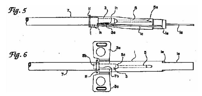
Figure 5 is a side view of a needle, winged needle hub (3), and slotted needle guard (1). '311 patent, col. 3, II. 4-6. In this depiction, the needle (5) remains retracted within the needle guard (1). <u>Id.</u> Figure 6 shows the same needle from above. '311 patent, col. 3, II. 7-10.
