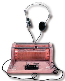
The crystal radio receiver, or crystal set, was one of the earliest forms of radio. Receiving power from radio waves rather than a typical battery, the crystal set was an easily made device.
